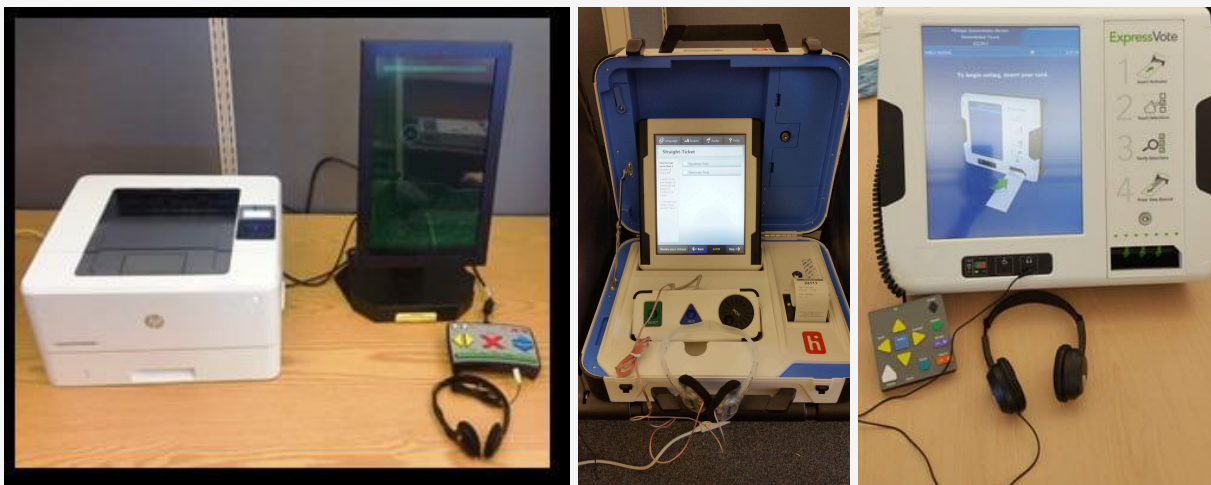
Figure 8: Accessible Voting Systems, known as the Voter Assist Terminal (VAT) in Michigan. Specific equipment is selected at the county level. A list of voting equipment by county can be found at https://mVIC.sos.state.mi.us/VotingMachineVendor/Index . From Left: Liberty Vote ImageCast ICX, Hart Verity Touch Writer, ES&S ExpressVote
